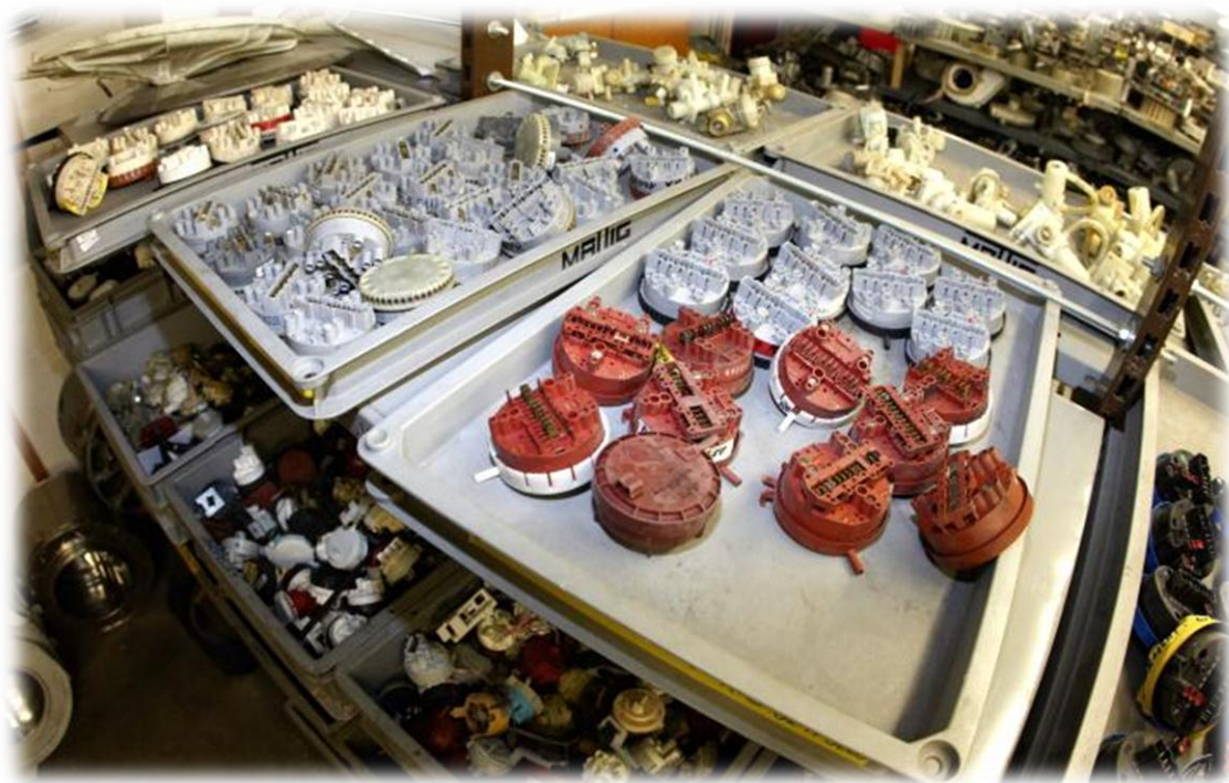
Figure 3: an array of pressure switches
